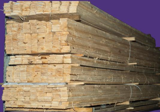
**Boards** — a type of lumber, whose width exceeds the thickness of two or more times. The thickness of boards — from 13 to 100 mm, width — from 50 to 260 mm. Boards with a thickness of 13 to 35 mm are called thin, the rest — thick. The wide sides of the boards are called faces, narrow — edges. By processing the side edges of the board are divided into edged, in which the edges are sawn off, and unedged, the edges of which are partially sawn or not sawn at all.
